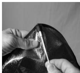
2. Small end of flex rod fits into corner pocket on the softbox tent.
