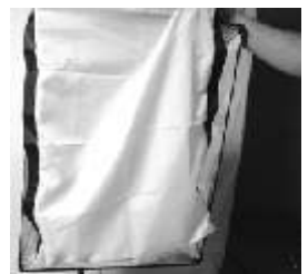
10. Attach the outer diffusion lens to velcro patches on the outer edges.
