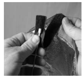
5. Insert the fourth rod into the pocket on the velcro strap.
