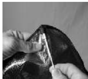
2. Small end of flex rod fit into corner pocket on the softbox tent.
