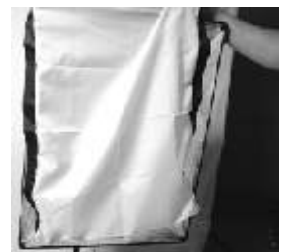
10. Attach the outer diffusion lense to velcro patches on the outer edges.
