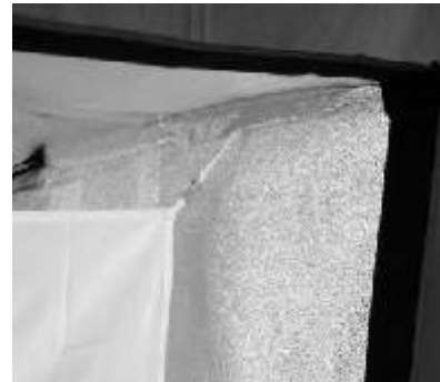
The inner lens is the first line of diffusion. It is made with translucent nylon and will not change the amount of light reaching the subject. It will change the texture of light when used. Experiment with and without.
