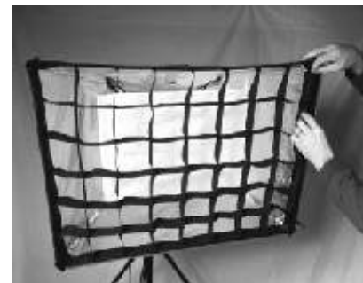
The grid lens will help direct the light flow to your subject. It will reduce the angle of glow by about 15°.
